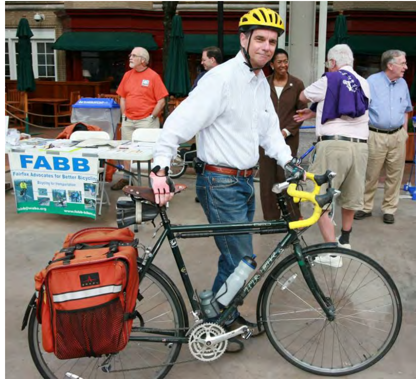
Classic Commuter Bike. Note storage bags, fenders, frame pump, twin headlamps
