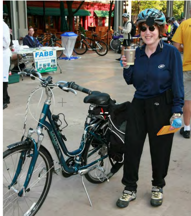
Janice Linkov-Johnson and her comfortable bike. Note step-through frame, high handlebars and forward pedals.
